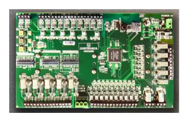
Las Vegas, NV (April 6, 2016) – Dortronics has expanded their line of Smart Interlock Controllers with today's introduction of the new highly versatile and economical 4800 Series here at ISC West (booth #1037). The new 4800 Series can be user configured in the field to accommodate up to five doors with ample flexibility for various input/output configurations.
